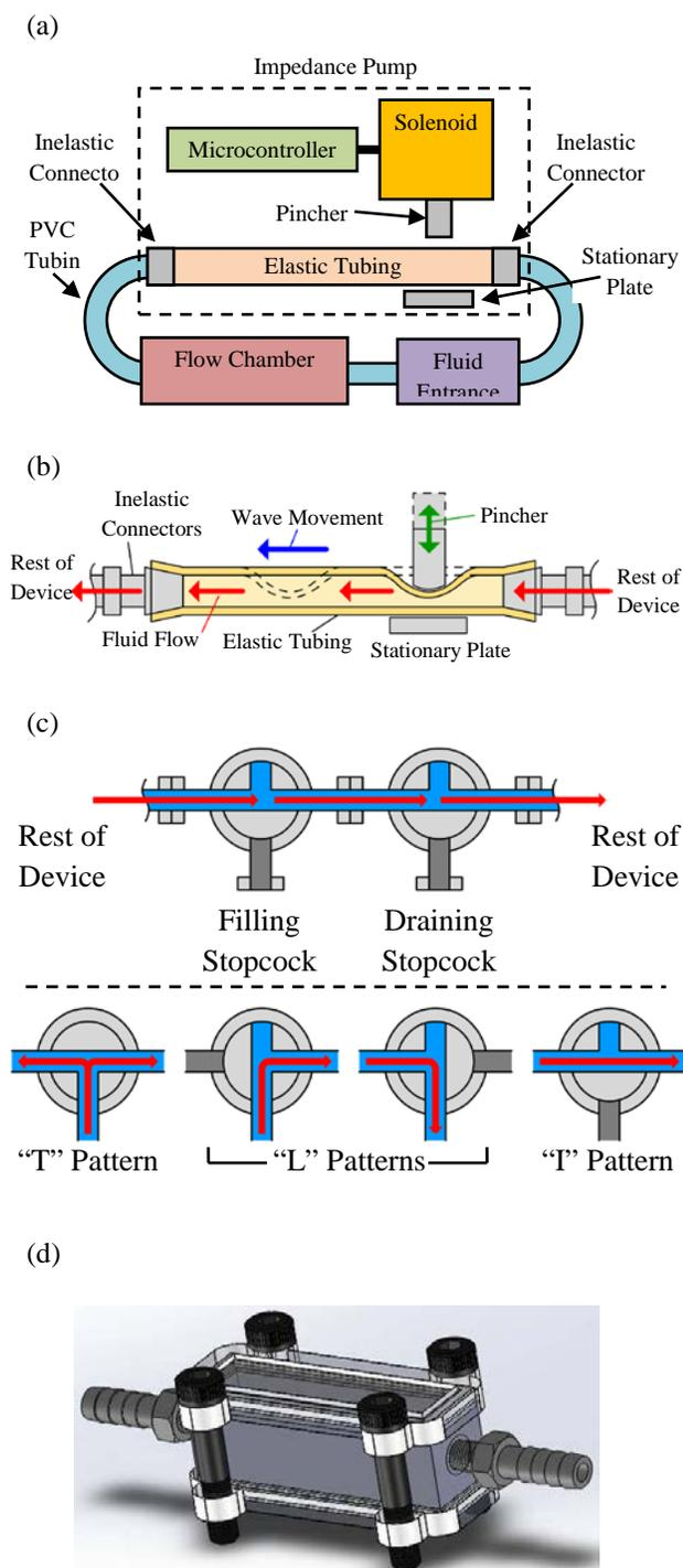
Figure 1. The schematic of the flow device. (a) Overview (b) An illustration of the principle behind the impedance pump. The illustration is not to scale. (c) The dual stopcock configuration that forms the fluid entrance. (d) 3D CAD drawing of the flow chamber used in this flow device.
