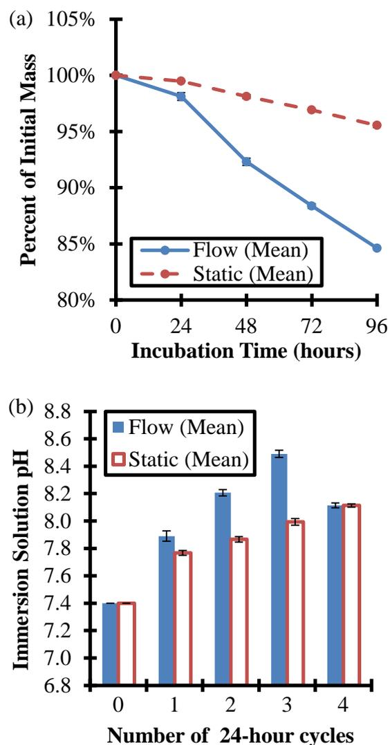
Figure 3: (a) Mass change of Mg samples in flow and static conditions (b) pH change of SBF working fluid in flow and static conditions at the end of individual 24-hour cycles (see text). Each data point in both graphs represents the mean of the three samples under the specified conditions. Note the incubation time does not include time spent UV sterilizing or drying overnight. The error bars represent  $\pm$  standard error of the mean ( $n = 3$  for each data series).
