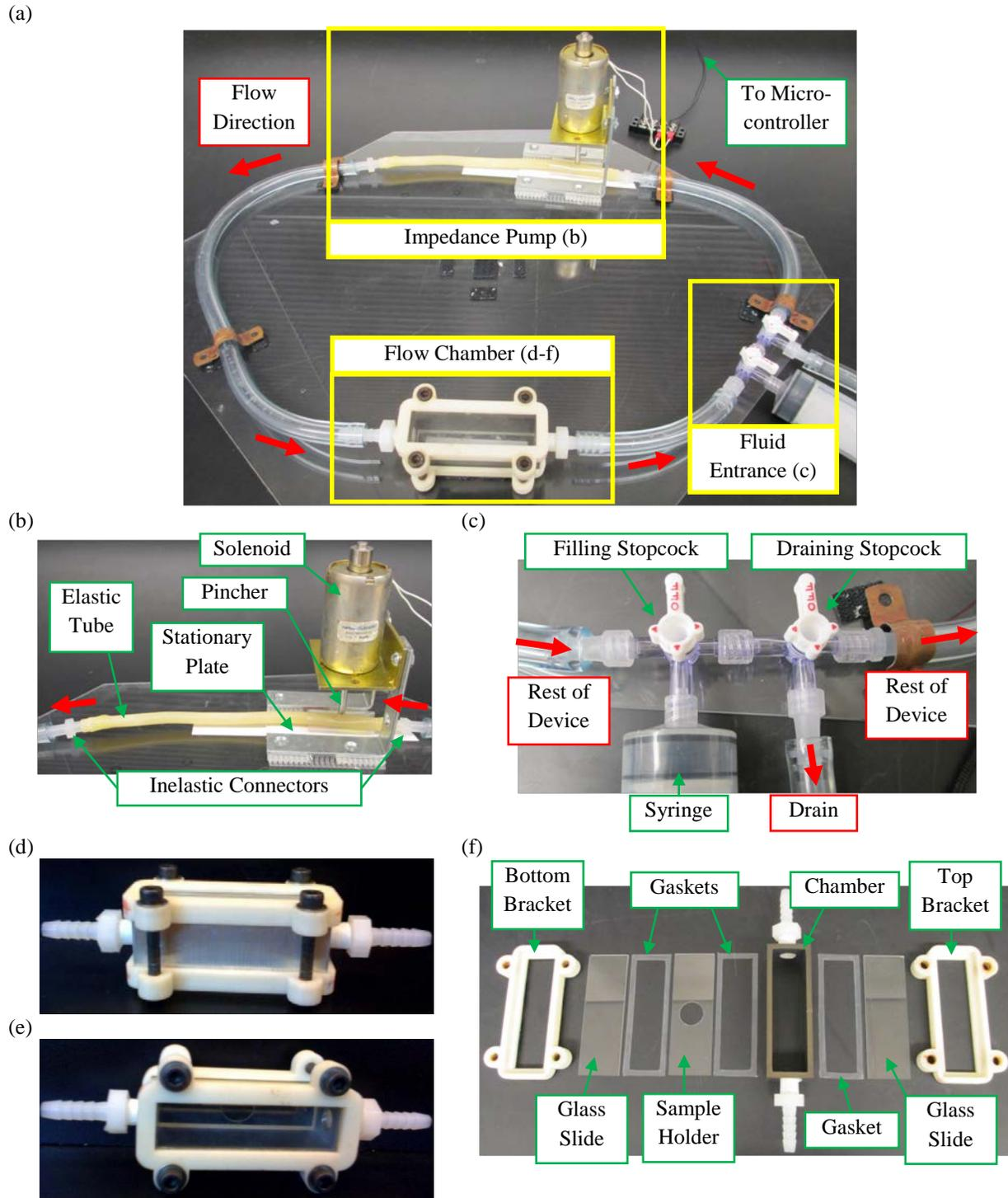
Figure 2: The implementation of the flow device: (a) Overview, (b) Impedance pump, (c) Fluid entrance, (d)
